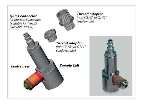
DSC74B Sample Cell - a two-pressure model for gas pressure and atmoshperic pressure furnished with inlet/ outlet valve and inlet/outlet connection for gas tubing
